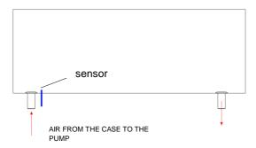
In most applications, locate the sensor near (but not directly in) the air input from the PMCG.
