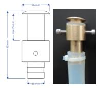
Typically, the PMCG is supplied with a silicone hose with an inner diameter of 5/8" - 16 mm. Connect to the hose using the fittings installed by the case manufacturer or with Preservatech's supplied air connectors (brass). For factory installed fittings we suggest a welded piece of metal pipe, 16 mm outer diameter and 30-40 mm long. For installing our brass fittings, a hole of 16 to 20 mm in diameter must be drilled in the case wall with a maximum wall thickness 1" - 26mm.
